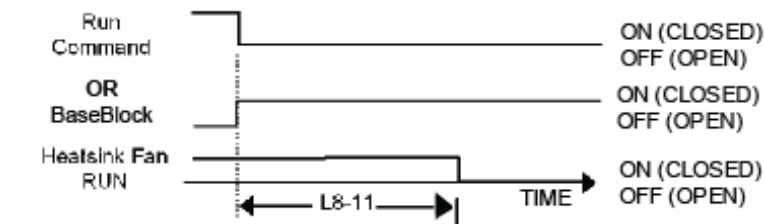
Figure 5.49 Heatsink Cooling Fan Operation Timing Diagram
